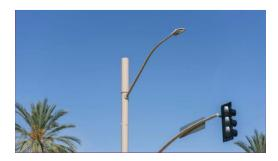
Small cells are low-powered, fiber-connected nodes that are usually located on existing structures like streetlights and utility poles.
