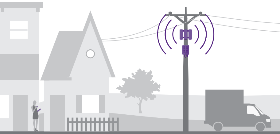
Small cells on utility poles
