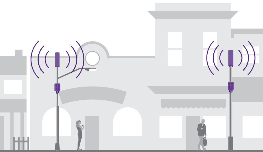
Small cells on streetlights and slimline poles
